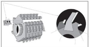
The Whisper Quiet II allows for the insertion of special adjustable inserts to produce plow cuts as well as profiles, shaping and molding simultaneously.
