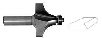
Ideal for rounding sharp corners and softening edges of furniture. Add a decorative touch by increasing the depth of cut until the shoulder produces a clean corner on the material. By changing the bearing you can convert a roundover bit to a beading bit.
